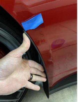
Then locate the driver side splashguard and starting at the top carefully apply it to the tape at the proper location previously marked, then apply even pressure to the splashguard as you adhere to the edge where the tape is.
