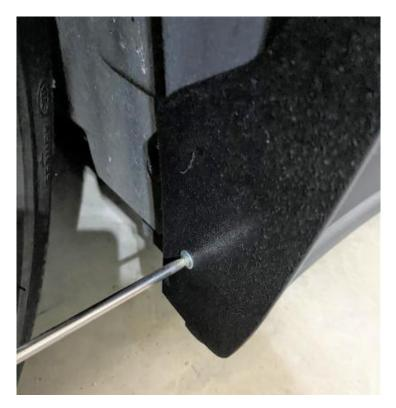
At this point locate the drill with the 1/16" bit and make a pilot hole on the wheel well using the provided hole in the splashguard as a guide.
