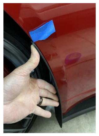
While holding the splashguard in place apply a temp piece of masking tape on the fender depicting the height of the splashguard
