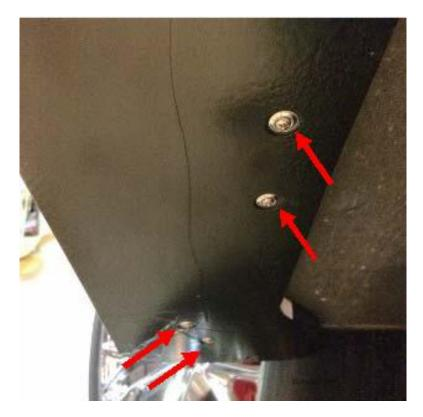
Under Car - Proceed doing the same installation to the (4) front screws, hand tight only. After installing all the 1  $\frac{1}{2}$ " long screws, the skirt should be able to hang between the front and rear screws.
