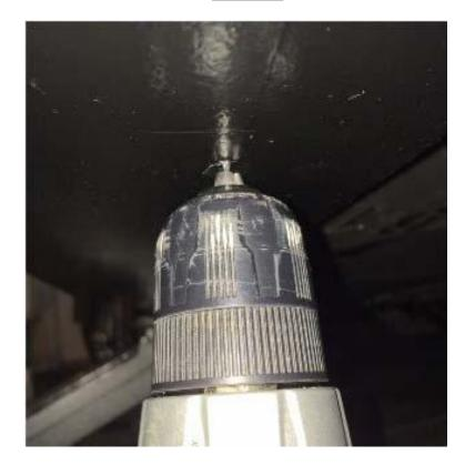
Under Car – Locate the (8) screw openings in between the front and rear stock screws already installed. Proceed to drill 1/16" dia pilot holes in each one of them. Remember the drill bit must only penetrate the rocker panel. See Pre-Installation on page 4.
