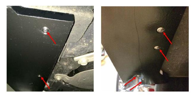
Once all the 1" screws have been installed (8), fully tighten the (2) rear and the (4) front 1  $\frac{1}{2}$ " screws from STEPS 3 & 4. This will conclude the screw attachments from the bottom of the car.
