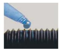
Locate the 1  $\frac{1}{2}$ " long screws [(2) rear and (4) front] and add few drops of Blue thread locker to each to help keep them in place.
