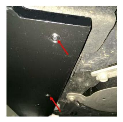
Under Car - With the skirt lifted up in place, align the skirt's (2) rear mounting holes with the (2) rear rocker panel screw openings. Proceed to install the 1  $\frac{1}{2}$ " long screws, only hand tight for now
