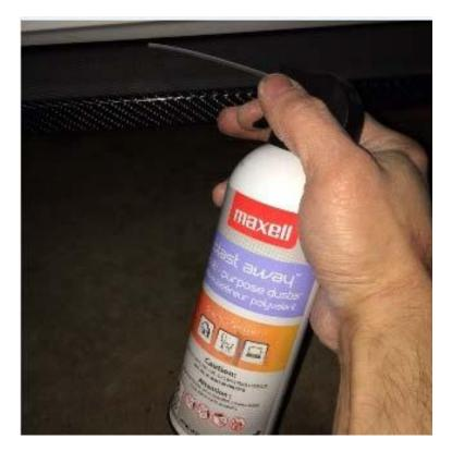
Once all the pilot holes are drilled ensure there is no debris left behind between the top of skirt and bottom of rocker panel. Blast some air near each opening to blow off any fiberglass residue.
