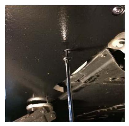
Under Car - Once the new (8) pilot holes from STEP 5 have been drilled proceed installing the 1" long screws, starting from the back towards the front. There should be (8) screws per skirt. Please note that the new screws will be making a new threaded connection through the rocker panel. For this reason it will be hard to turn the screws. Fully tighten them all up by hand. (no power tools).
