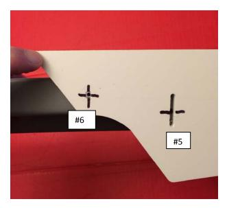
Proceed with marking the stage 2 wickerbill screw holes #5 and #6 locations. If your piece is already wrapped use masking tape to locate holes. This is necessary to be able to see locations through the Stage 3 piece
