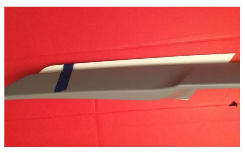
Ensure the space between the top of the wickerbill and the top surface of the spoiler Is consistent and even
