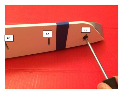
Using the 1/16" drill bit cut first hole and attach screw #1, hand tight but secured
