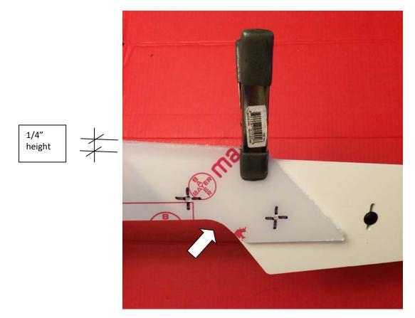
Using the spring clamps, hold the Stage 3 wickerbill in place. Ensure the center piece is even on both sides of the spoiler using the bottom curved inside edge as a guide. You should have about 1/14" space above the Stage 2 wickerbills. Proceed marking on the Stage 3 wickerbill screw holes #5 and #6 on both sides.
