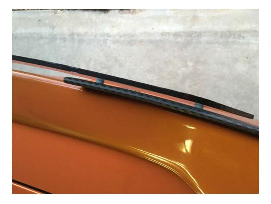
Once screw hole #5 and #6 are cut on both sides of the Stage 3 wickerbill, and before final installation to the Z51 spoiler, install the provided nylon spacers between the Stage 3 and the Stage 2 wickerbills. This ensures that water and debris don't get caught in between both pieces. Temporarily hold the spacers in place while attaching the Stage 3 piece to the Stage 2 wickerbills. Do this on both Left and Right sides.
