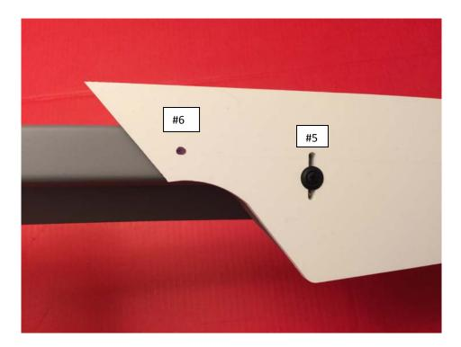
With screw #1 and #5 tightened, mark screw #6 hole. This should be in the middle of the vertical piece of the Z51 spoiler. Using the 3/16" drill bit cut the hole on the wickerbill. IMPT. DO NOT ALLOW the 3/16" TO PENETRATE THE SPOILER. ONCE THE 3/16" HOLES IS CUT THEN SWICTH TO THE 1/16" DRILL BIT TO MAKE HOLE IN THE SPOILER.
