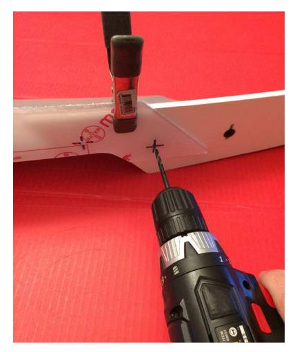
Using the 3/16" drill bit, cut holes #5 and #6 in the Stage 3 wickerbill from previous step. If you prefer you can do this step on a flat horizontal plane. Do both sides of the Stage 3 wickerbill. After cutting holes, remove the Stage 3 wickerbills protective film from both sides.
