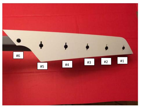
Once screws #1, #5 and #6 are secured, proceed with the 1/16" bit and cut holes for #2, #3 and #4 screws. Attach all screws and tighten all screws until secured on the Z51 spoiler. Ensure that only enough force is applied to each screw to cut into the Z51 spoiler but not too much that it strips the threaded connection the screw made.
