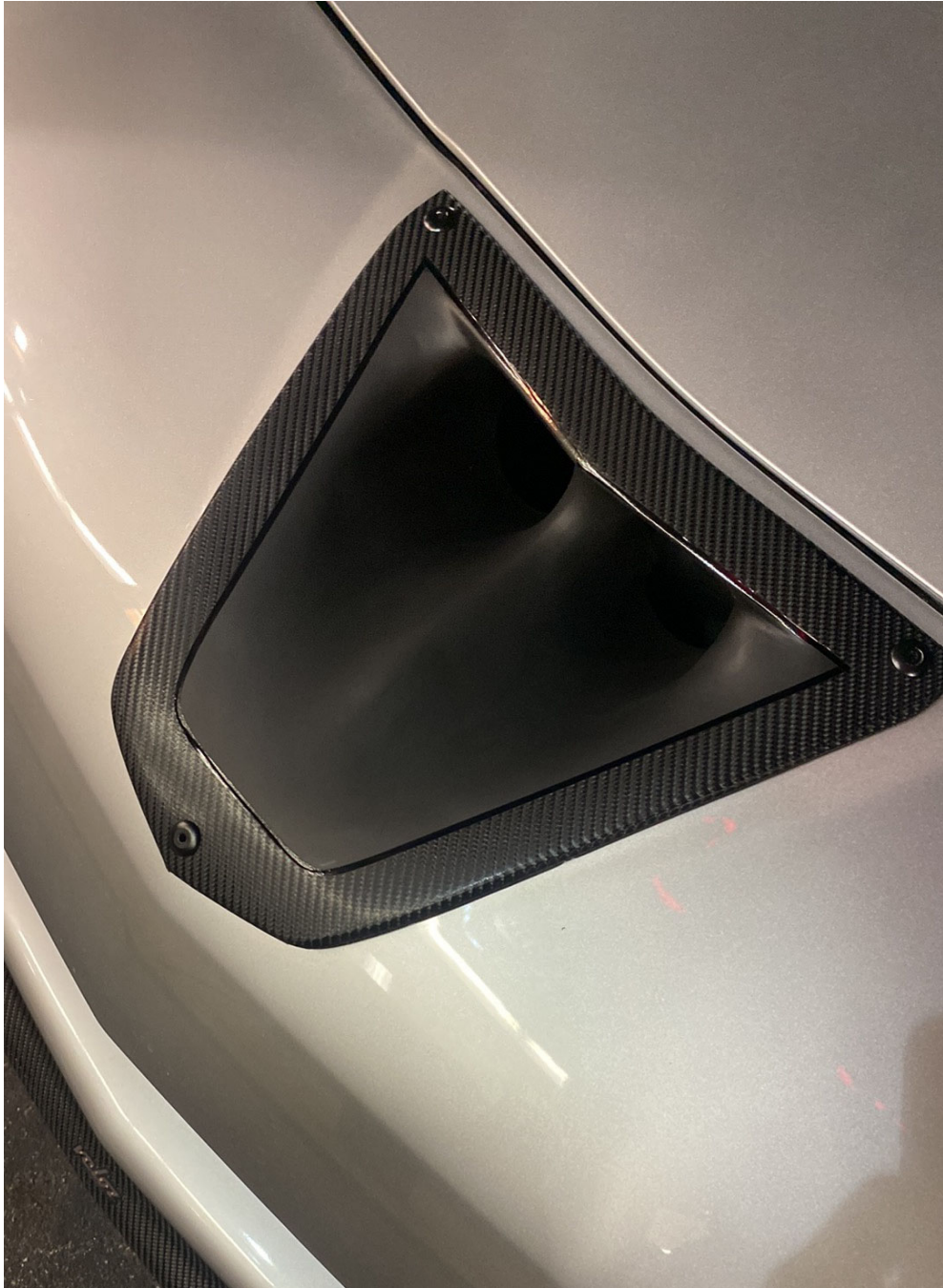
Complete look of the scoop with rivets.
