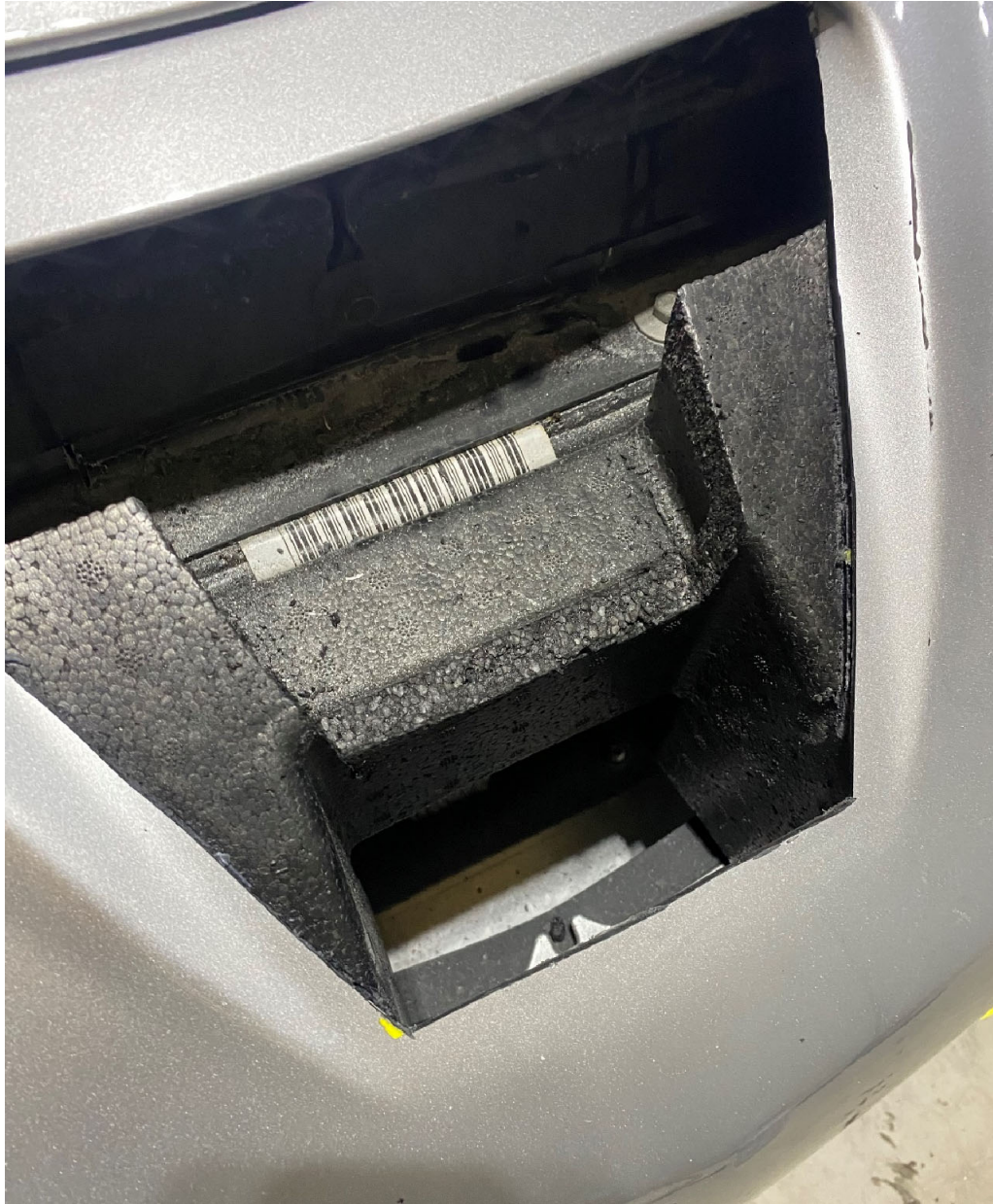
Center section of foam removed.
